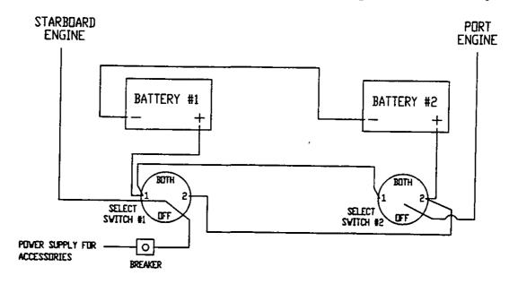
In an emergency situation when neither battery will start the engine(s) the select switches allow you to combine the power of both batteries by selecting BOTH. The switches should be returned to either the #1 or #2 position after the engines are started to allow each battery to be charged.
