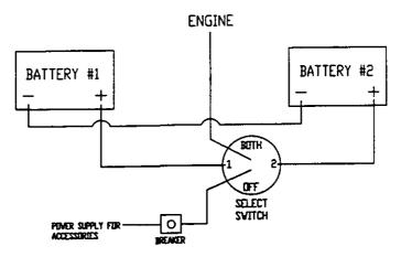
On twin engine boats with two select switches, a switch should be connected to each engine. Either battery may start either engine by selecting position #1 or position #2 on the switches. In normal use select position #1 on one switch and position #2 on the other so that both batteries will be charged simultaneously.
